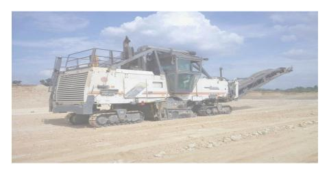
Surface Miner is a machine which cuts the in-situ rock in thin vertical or horizontal slices without drilling and blasting, the output size being less than 150 mm
